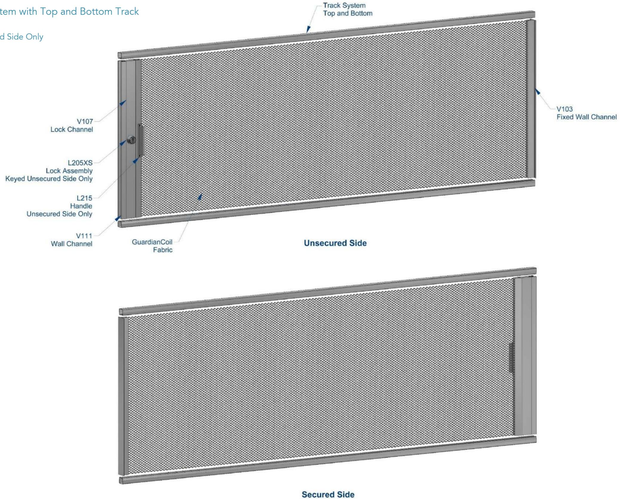
Right End Opening Security System with Top and Bottom Track
