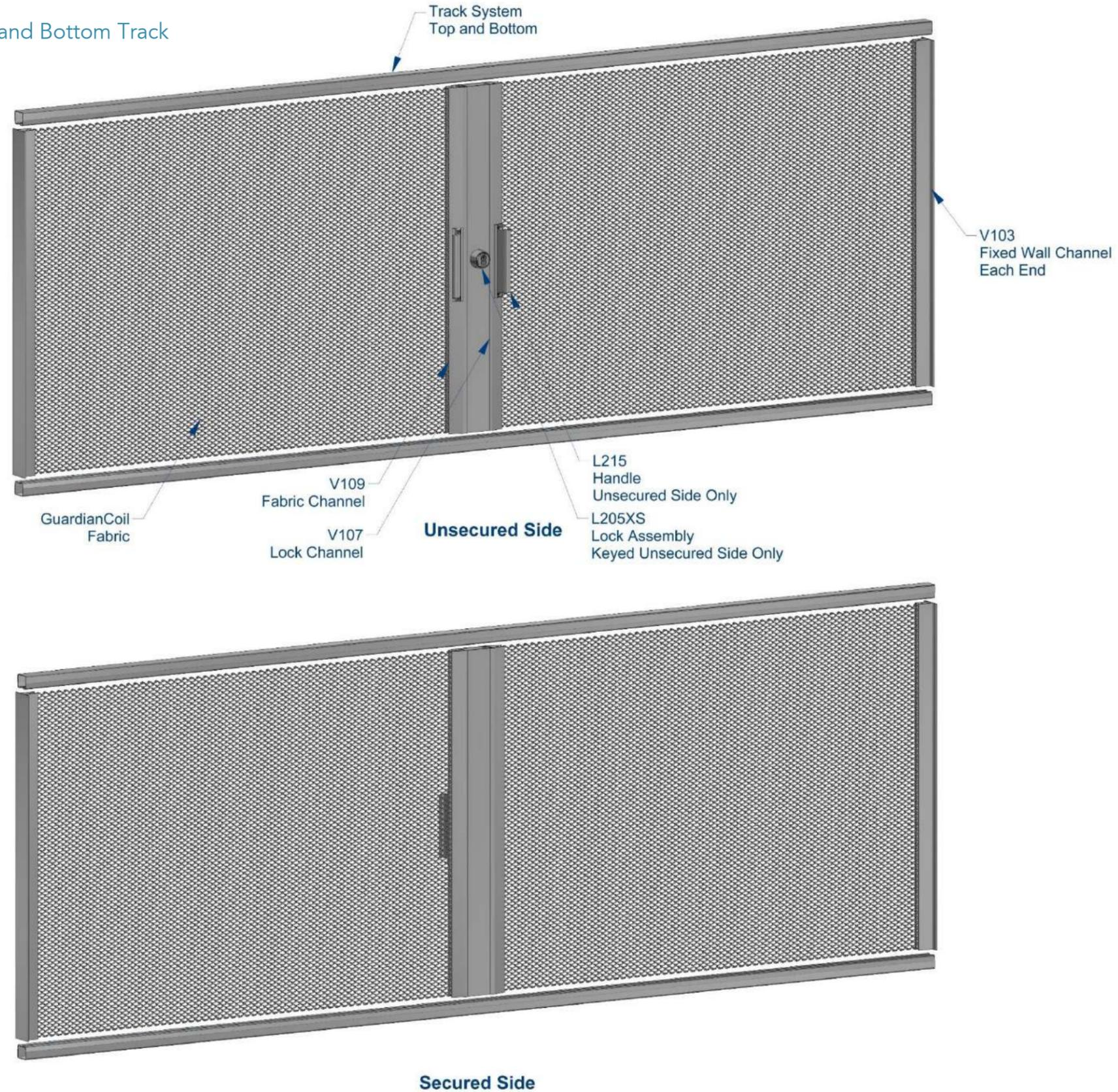
Left and Right End Opening Security System with Top and Bottom Track
